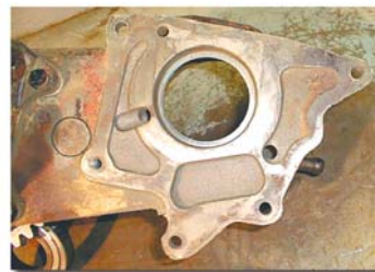
Small Hole transfer case (3-1/8")
