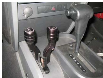
Jeep JK console (right) with the RubiCrawler twin stick shifter installed. The shifter knobs in this photo are the upgraded aluminum knobs P/N 42R650.
