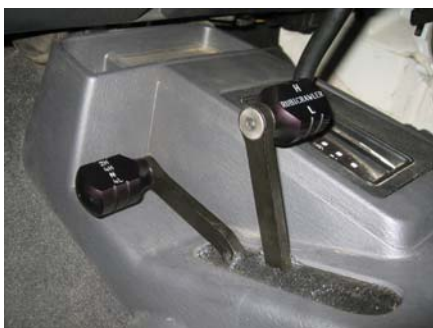
Jeep JK console (right) with the RubiCrawler twin stick shifter installed. The shifter knobs in this photo are the upgraded aluminum knobs P/N 42R650.
