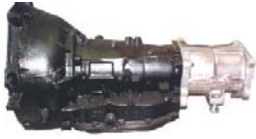
AOD transmission with 50-8403 adapter
