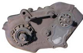
NP205 T/C figure-8 bolt pattern
