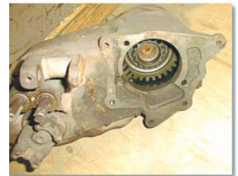
Large Hole transfer case (4")
